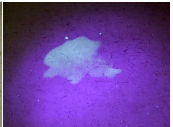
Four F Milk Under Bactiscan ATP Reading = 17,023 RLU's
